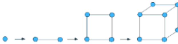
Figure 11: Principle of the B-rep approach in the geometry definition.
