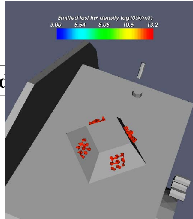
Fast In + density log 10 (#/m 3 ) – isosurfaces at 11 and 12.5
